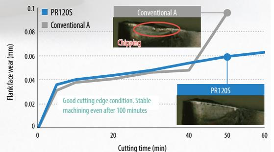
Cutting conditions : Vc = 150 m/min, ap = 1.0 mm, f = 0.08 mm/rev,
