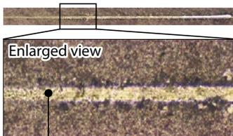
Peeling load (Lc1) (Internal evaluation)
